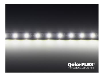
**QolorFLEX LED Tape, Natural White, 12V Indoor** (P/N 3528-12-NW-60-5-20-1) is an economically priced interior grade LED tape with a medium/low output (330 lumens/metre) brightness. Intended for applications where high light output is not required, the natural white colour (4100°K) is ideal for use where good colour rendition is needed. Each LED tape comes with wiring leads on both ends and durable 3M adhesive backing. It is available in full five metre reels and sample strips.
